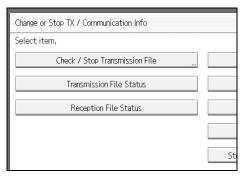
The list of stored files being transmitted or waiting for transmission appears. To display only the files being sent, press [Files under TX].
